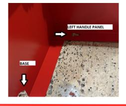
STEP 5. RIVET SIDE PANEL TO BASE X 2
